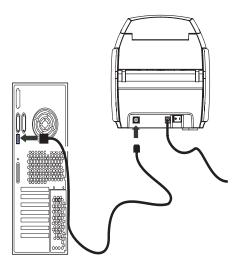
**5.** Attach USB cable to printer and computer.
